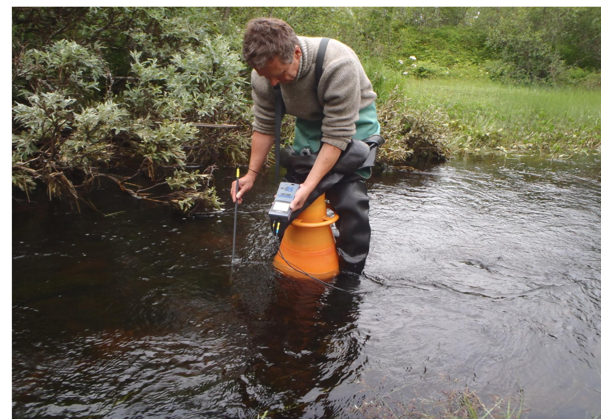
Measuring redox potential from river sediment
